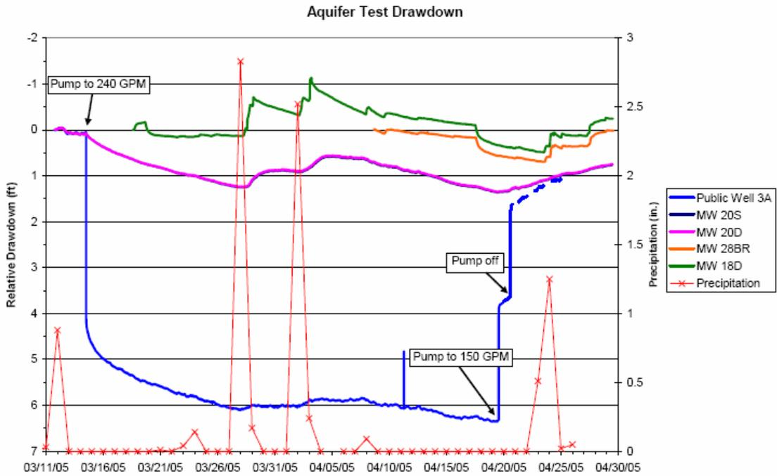
**Figure 5:** Drawdown curves obtained from pressure transducers. Precipitation is also plotted. The origin of the anomalous point in Public Well #3A on 4/10/05 is unknown. It may have been related to a very short pump disruption.
