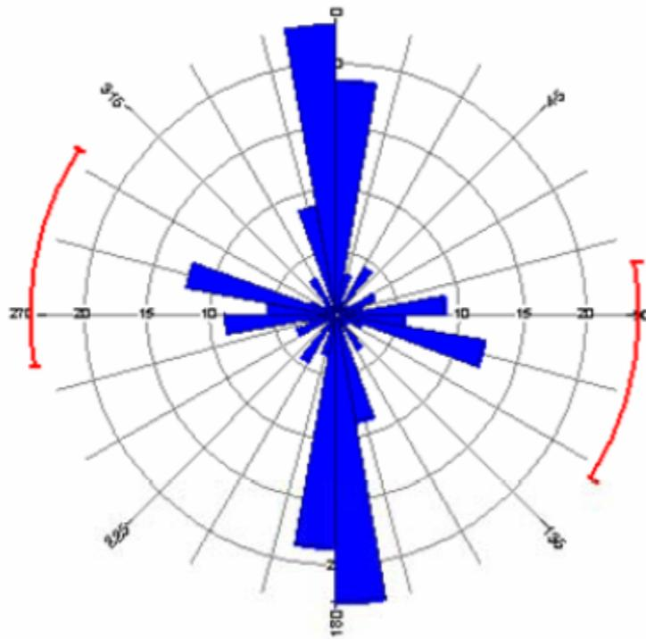
**Figure 7:** Average fracture strike for all field measurements
