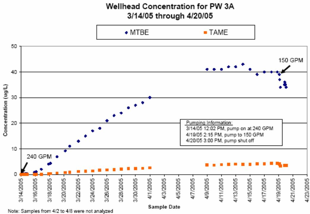
**Figure 6:** Concentrations of MTBE and TAME at the wellhead from the start of the aquifer test through the end. Notice the apparent steady state at 43  $\mu\text{g/L}$  for MTBE and the drop when pump rate changed.
