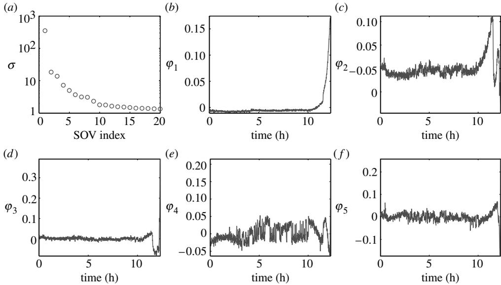
Figure 11. Fatigue damage identification: (a) largest 20 SOVs of the truncated tracking matrix; (b–f) the five SOC<sub>s</sub> corresponding to the largest five SOVs.
