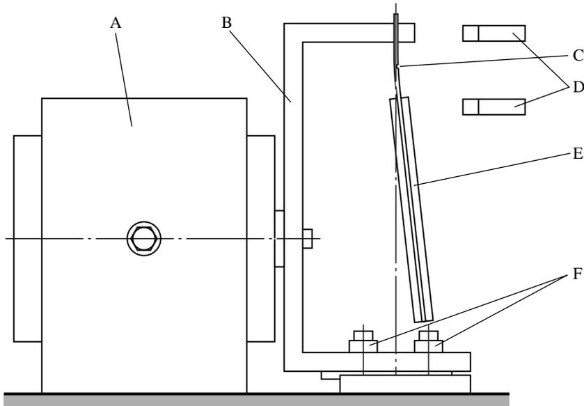
Figure 7. Schematic of the experimental apparatus: A, electromagnetic shaker; B, frame; C, notch in the beam; D, laser vibrometers; E, steel beam with stiffeners; F, permanent/electromagnet stacks.
