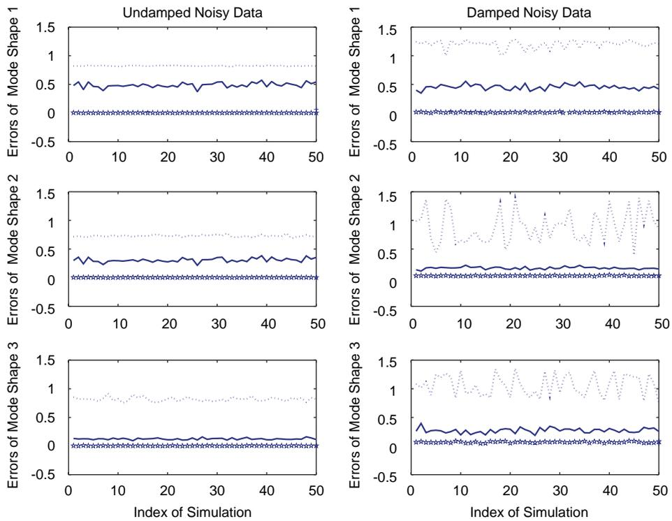
Fig. 7. Comparison of the mode shape extraction in the noisy environment. Left column contains the results for the undamped case. Right column is composed of the results from the damped case. The solid lines represent the results from AMUSE. The dotted lines are from ITD method. Stars (☆) are for SOBI.
