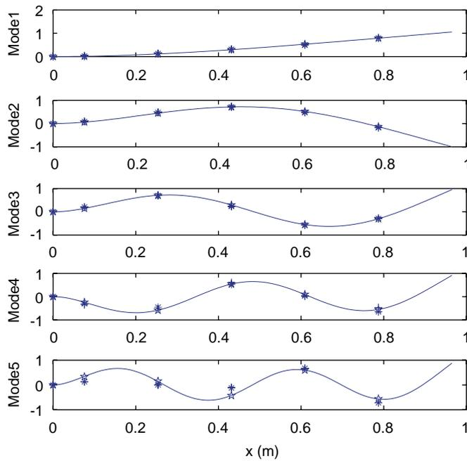
Fig. 12. Comparison of mode shapes from SOBI, ITD, FEA and Euler–Bernoulli beam theory. Continuous lines represent mode shapes from beam theory, “\*” represent results from SOBI, “+” are from ITD analysis and “★” are from FEA.
