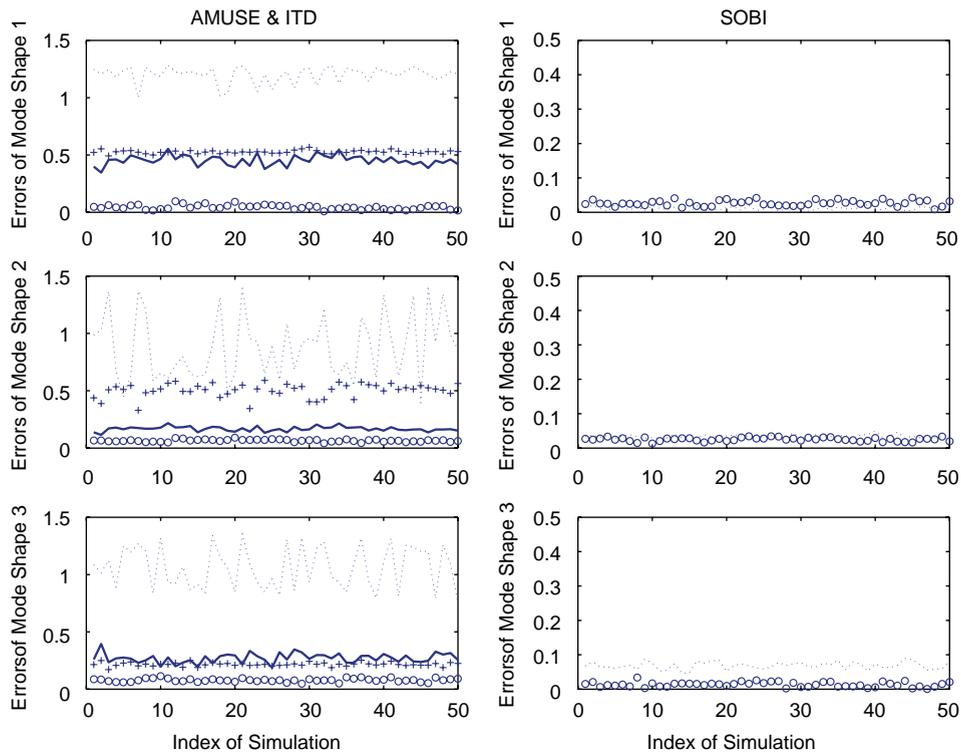
Fig. 8. Comparison of the mode shape extraction before and after PCA preprocessing. Left column are for AMUSE and ITD. The solid lines represent the results from AMUSE without PCA, the dotted lines are from ITD method without PCA, circles (o) and pluses (+) are from both methods after PCA, respectively. Right column is for the case of SOBI. The dotted lines represent the results from SOBI without PCA. Circles (o) are for the results of SOBI after PCA.
