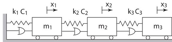
Fig. 5. A three-degree-of-freedom damped vibration system.
