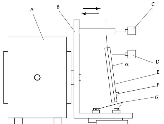
Figure 1. Experimental apparatus: (A) electromagnetic shaker, (B) sliding frame, (C) laser vibrometer ch1, (D) laser vibrometer ch2, (E) cantilever beam, (F) Accelerometer, and (G) permanent/electromagnet stacks.
