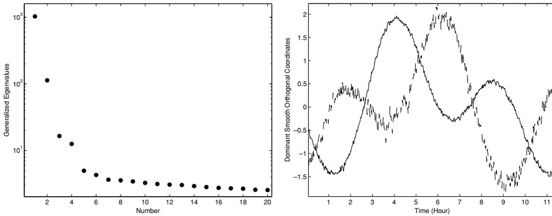
Figure 5. Left plot: first 20 largest generalized eigenvalues of Equation (7) for a base experiment. Right plot: the SOCs identified from the time series. Solid line shows tracking modes corresponding to the largest eigenvalue, and dashed line corresponds to the second largest eigenvalue.
