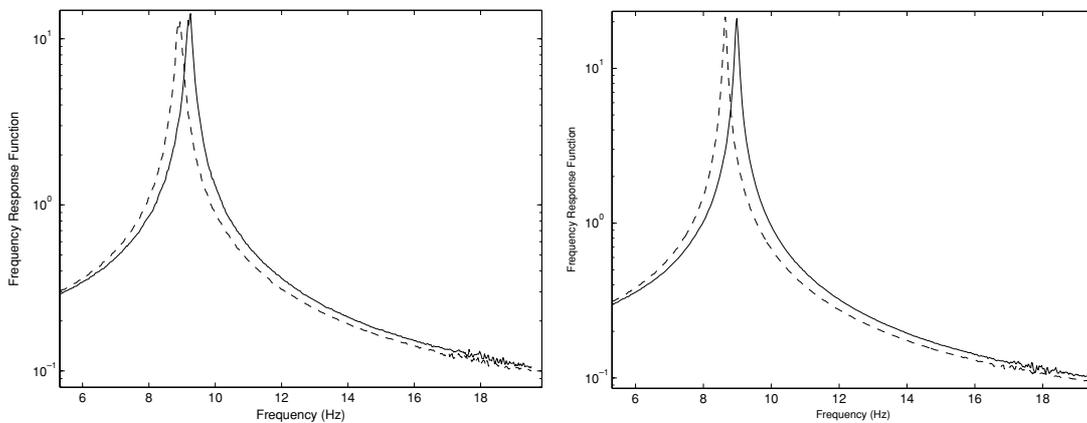
Figure 3. Frequency response functions for small oscillations in front (left plot) and back (right plot) energy wells. Solid line: 1 V on the stack and dashed line: 19 V on the stack.
