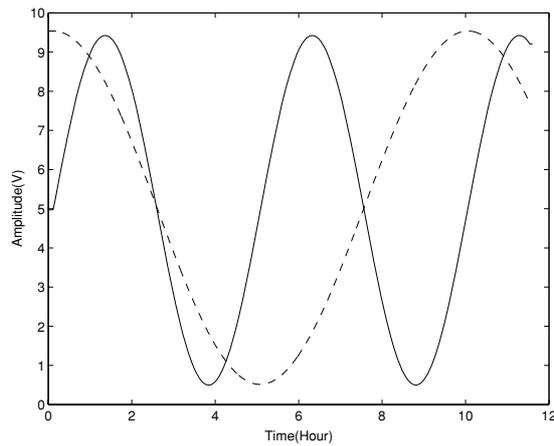
Figure 2. Voltage of the outputs of power supply. Solid line describes the voltage supplied to the front electromagnet, and dashed line to the back stack.
