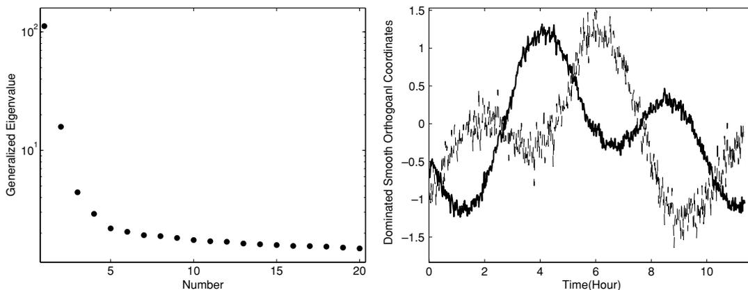
Figure 8. Left plot: first 20 largest generalized eigenvalues using the data collected from the accelerometer. Right plot: the SOCs identified using the data collected from the accelerometer. Solid line shows tracking modes corresponding to the largest eigenvalue, and dashed line corresponds to the second largest eigenvalue.
