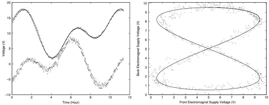
Figure 6. Left plot: two combinations of the two input voltages ( $v_1 + v_2$  solid line and  $v_1 - v_2$  dashed line), and the scaled first two SOCs (dots). Right plot: phase trajectory of the power supply terminal voltage (solid line) and the identified trajectory after affine transformation (dots).
