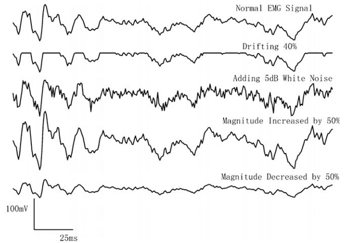
**Figure 2.** Examples of 200 ms of simulated EMG signals with different distortions.
