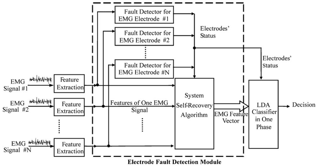
**Figure 1.** Block diagram of the EMG pattern recognition system with a sensor fault detection module.
