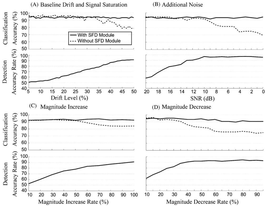
**Figure 4.** The classification accuracy of the system with and without the sensor fault detection module for increasing signal distortion levels (upper panel of each subplot) and the detection accuracy rate of the designed sensor fault detector for increasing signal distortion levels (lower panel of each subplot). These representative results were derived from the EMG signals recorded from the rectus femoris of TF1.
