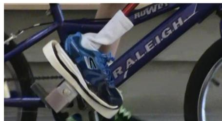
**Figure 5. Testing and documenting revised 'slipper' designs to accommodate the prosthetic leg and foot angled positions to improve balance and power.**
