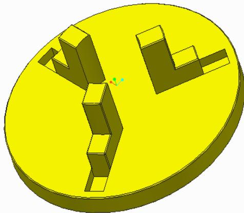
Fig 5- Pro-e model of Bottle bottom holder
