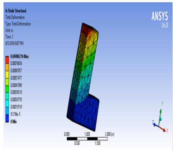
Fig 11- Result of total deformation analysis of chuck of bottle bottom holder using ANSYS.
