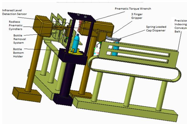
Fig 1- Pro-e model of assembly of Capping System
