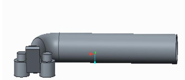
Fig 3- Pro-e Model of Spring Loaded Cap Dispenser
