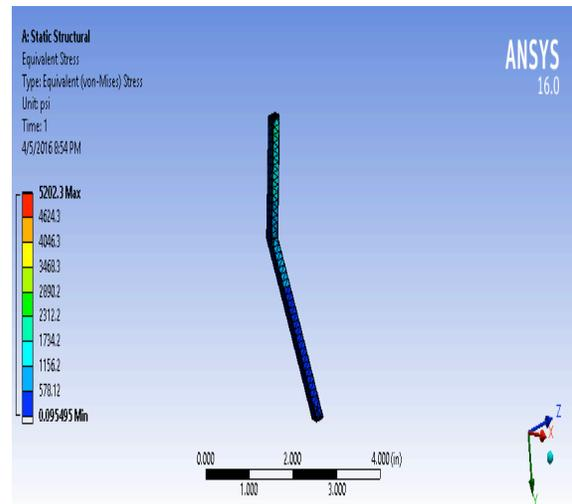
Fig 8- Result of equivalent stress analysis of finger of self-centering gripper using ANSYS
