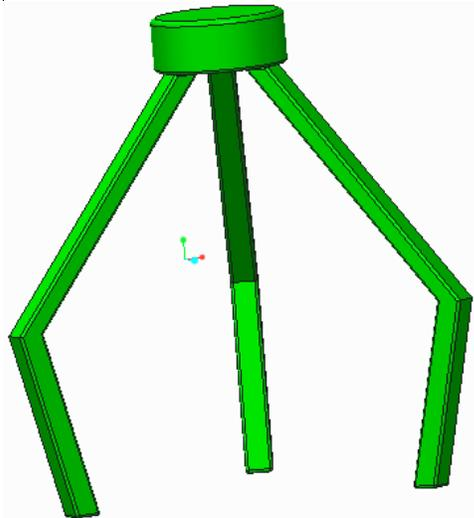
Fig 4- Pro-e model of three finger self-centering gripper
