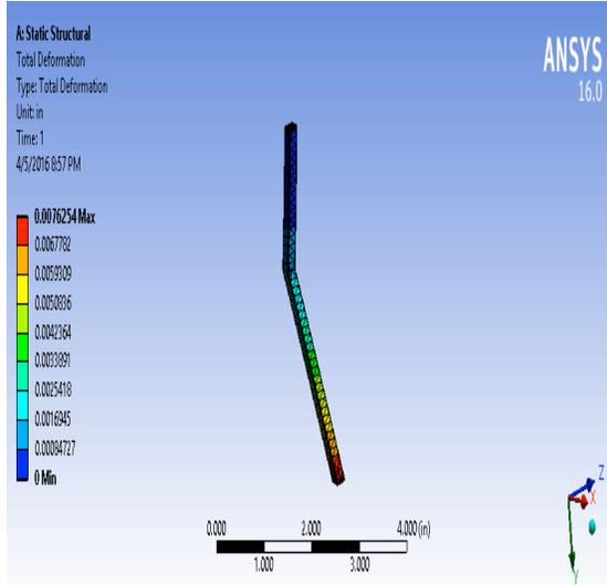
Fig 9- Result of total deformation analysis finger of self-centering gripper using ANSYS.
