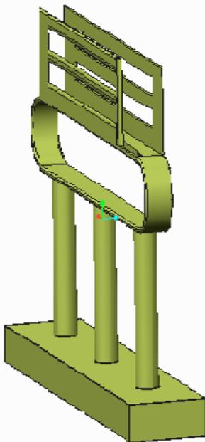
Fig 2- Pro-e Prototype of Precision Indexing Conveyor System
