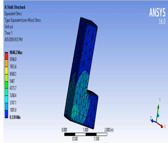
Fig 10- Result of equivalent stress analysis of chuck of bottle bottom holder using ANSYS.
