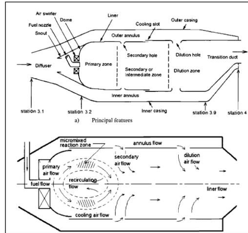
Figure 6 A detailed look at the combustor components [5]
