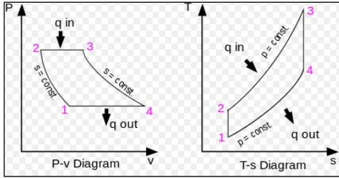
Figure 2 Graphs depicting pressure-volume and temperature-entropy changes during the four stages for this system
