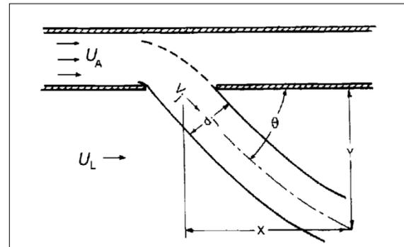
Figure 8 A depiction of the fluid flow from the annulus region into the liner region [5]
