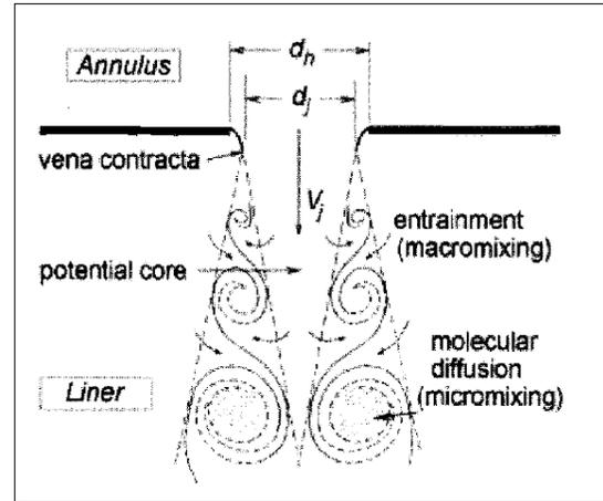
Figure 7 A depiction of the air jets forming inside the flame tube [5]
