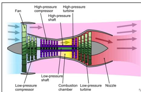
Figure 3 various components of the standard jet engine [3]
