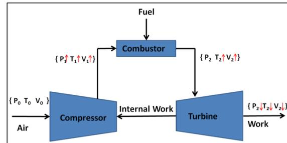
*Figure 1 Air-standard Brayton cycle depicting the necessary components[3]*
