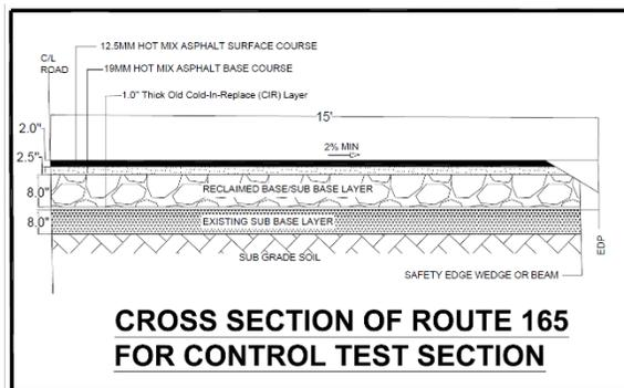
Figure 3 Cross Section of Control Test Section on Route 165
