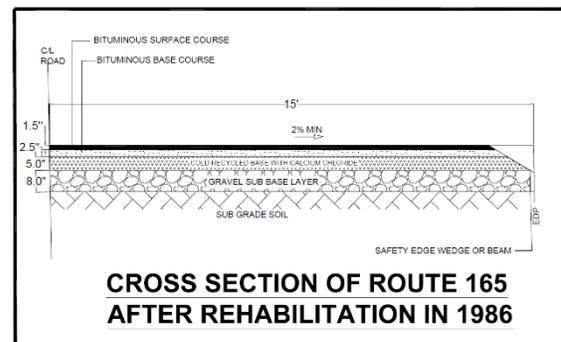
Figure 2 Cross Section of Route 165 after Rehabilitation in 1986
