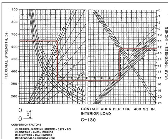
Figure 4 Rigid pavement thickness design C-130 (Navy)
