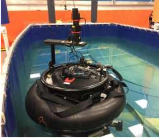
Figure 1. Dynamic positioning platform, in test tank, with 3 LIDAR sensors offset by 120^\circ
