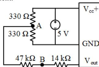
Figure 2: Circuit design of a hall sensor with relative output readings across node A and B.
