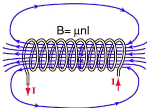
Figure 1: Magnetic field of a solenoid.  $\mu$  = magnetic permeability.  $N$  = turns.  $L$  = length of solenoid.
