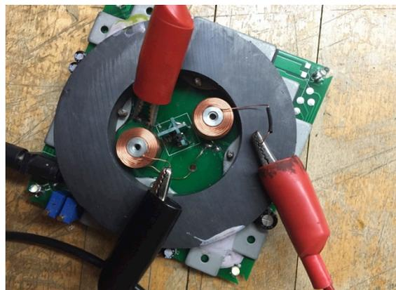
Figure 5: Measuring the current through the solenoid using the second method.
