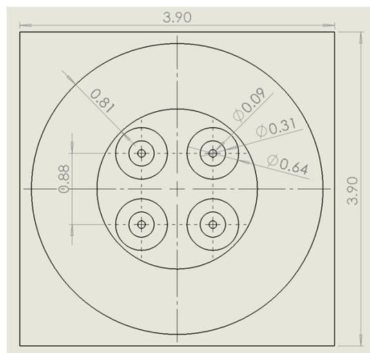
Figure 4: Measurements of the magnetic base and the geometry of the solenoids.
