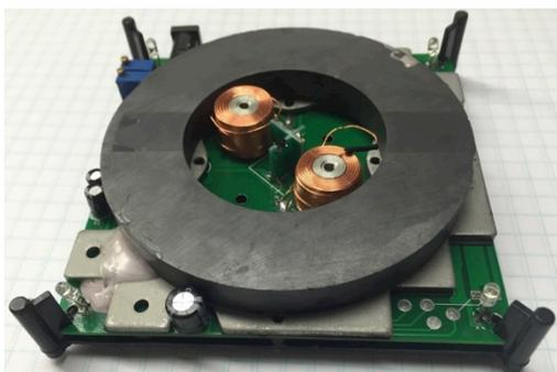
Figure 3: Layout of Levitron magnetic base and solenoids.
