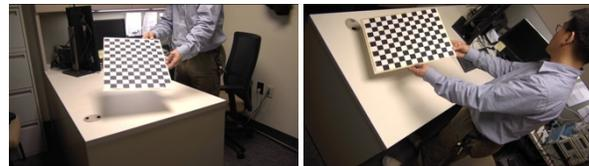
Figure 7: Snapshot of camera calibration using a standard calibration pattern.
