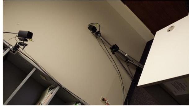
Figure 5: Testbed configuration using a flat table and two synchronized cameras. Left-view camera on the tripod, right-view camera on the clamp.
