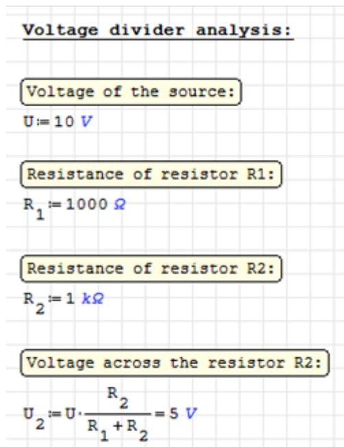
Figure 2. Numerical evaluation of the output voltage.
