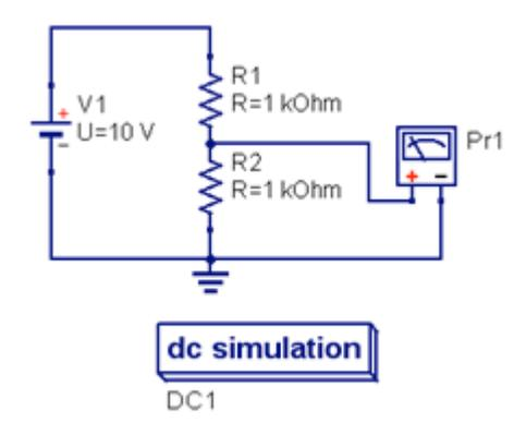
Figure 3. Simulation circuit.
