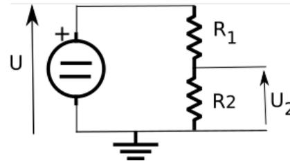
**Figure 1.A voltage divider circuit.**
