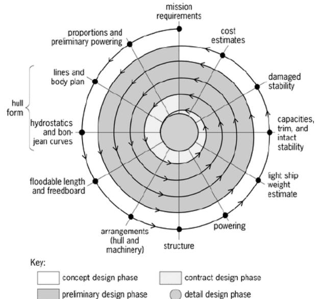
**Figure 1:** Evans' design spiral for ship design, first introduced in 1959.
