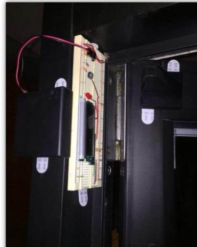
Figure 2: Door Opening Counter Installed
