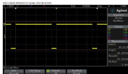
Figure 7: sample waveform indicating a duty cycle of 88.5%.
