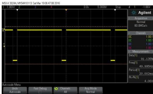
Figure 8: sample waveform indicating a duty cycle of 91.1%.
