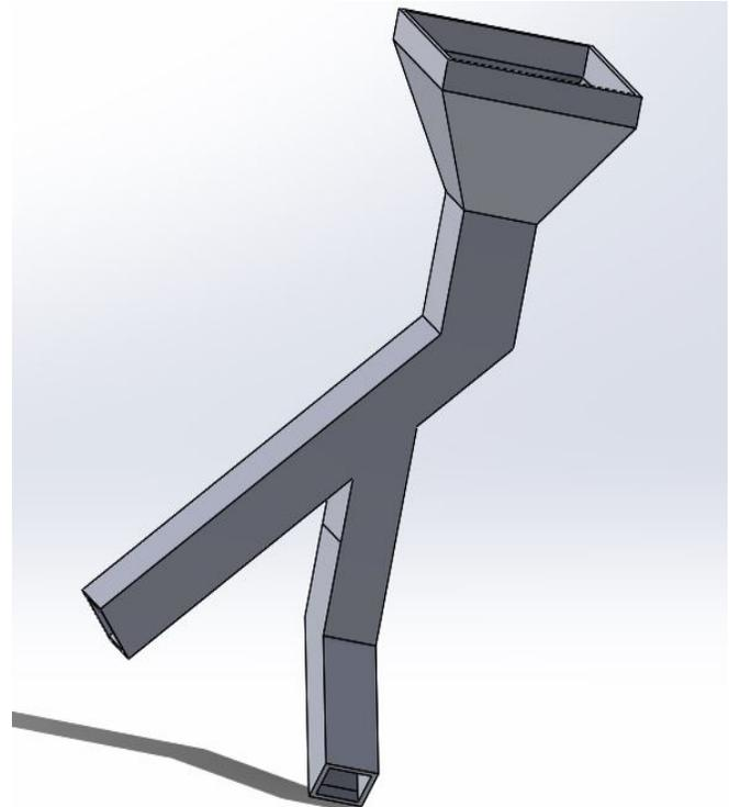
**Figure 1:** The above Solidworks design of the square funnel module leading into the duel shoot design
