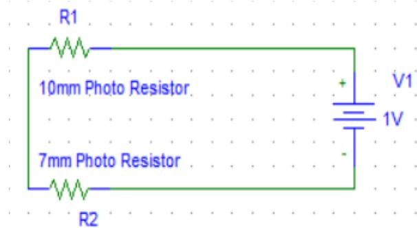
**Figure 2.** The diagram of the photo resistor schematic was drawn using Pspice Design Manager. Resistor R1 represents the 10mm diameter photo resistor, while R2 represents the 7mm diameter photo resistor.
