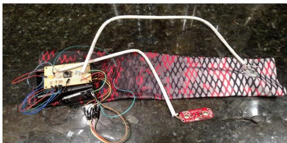
*Figure 5. The prototype of the system with sensors, LEDs, SD card, and push button.*
