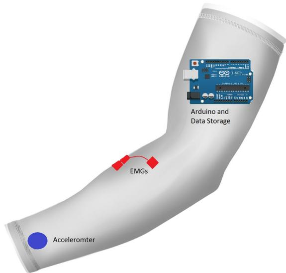
Figure 4. Conceptual sleeve design
